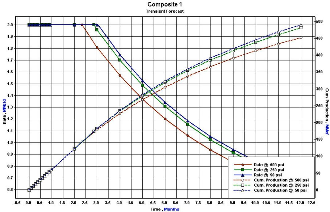
In an effort to determine the sensitivity of the formation to backpressure, I have projected the production against three different pressures 500, 250 and 50 psi. Obviously the lowest curve is the highest backpressure and vice versa. In this case it appears that the well can flow an additional 200mcf/d by lowering the pressure from 500 psi to 50 psi. Adding compression can lower the backpressure.
